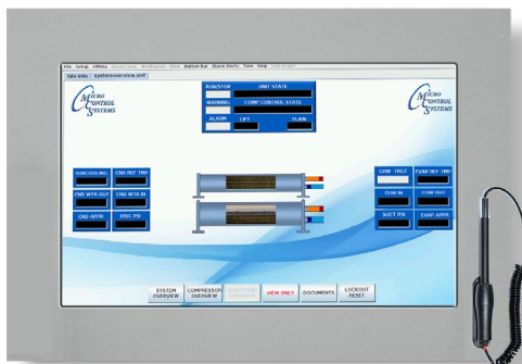
EVAPORATOR CONDENSER OVERVIEW SCREEN
